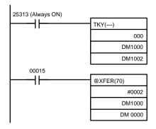
The 10-key information input to IR 000 using TKY(—) is converted to BCD and stored in DM 1000 and DM 1001. Key information is stored in DM 1002.
